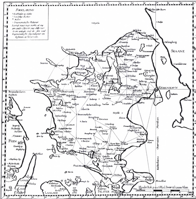
The network of geodetic triangles around Sealand measured by Thomas Bugge and Ole Wessel 1765-1771. – From Bugge's description of his cartographical methods, published in Danish at Copenhagen in 1779.
